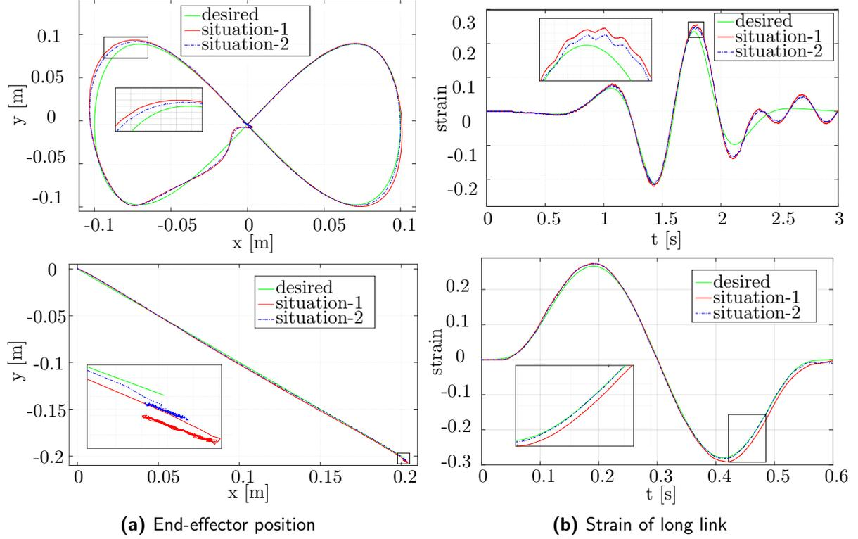
**Figure 2.** Experimental comparison of two model for nonlinear and linear trajectories
