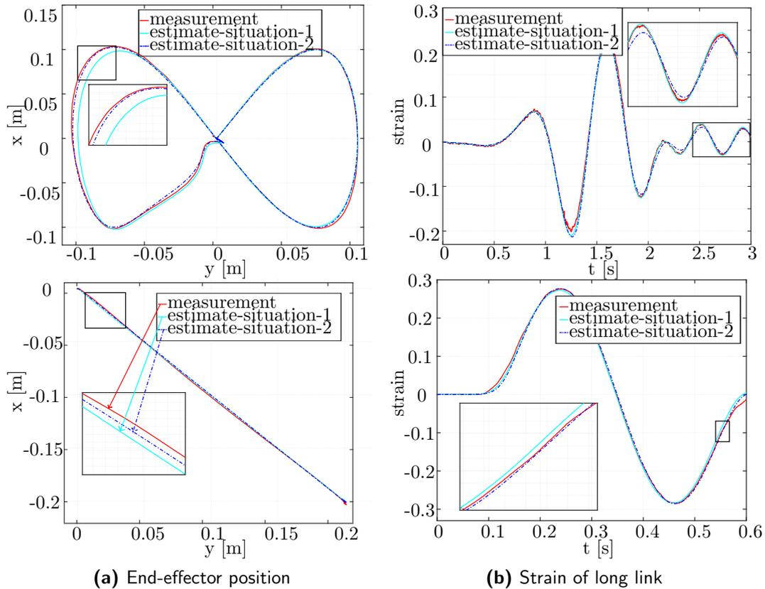
**Figure 3.** Compare measurement results of the camera and strain gauge with observer results based on the model situation-1 and situation-2 for the linear and nonlinear trajectories
