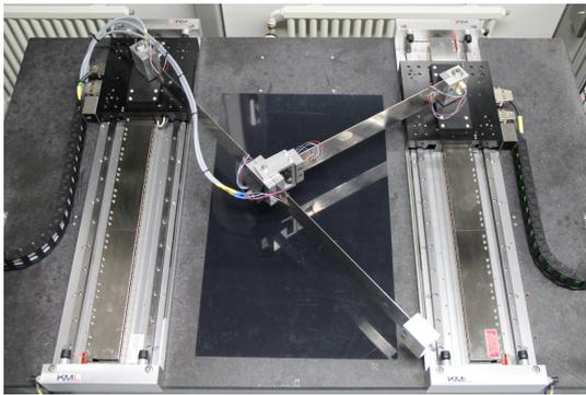
(a) Mechanical setup of the lambda manipulator
