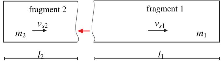
Figure 1. Fragments after spallation
