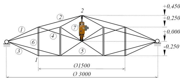
**Figure 1.** Section view of cable dome in Levy form with geometry with described basic members: (1) and (2) rigid cables, (3) and (4) diagonal cables, (5) hoop cables, (6) vertical struts and (7) active member.
