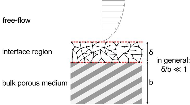
**Figure 1.** Conceptual scheme of the novel coupled model consisting of a free-flow region (Stokes), an interface region (pore-network model) and the bulk porous medium (Darcy).
