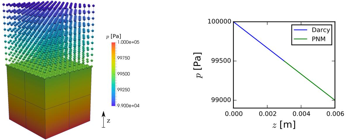
**Figure 2.** Exemplary coupling of a pore-network model (interface region, top) and a REV-scale model (bulk domain, bottom). The plot on the right indicates the continuity of the pressure itself and its identical gradient within the two domains.
