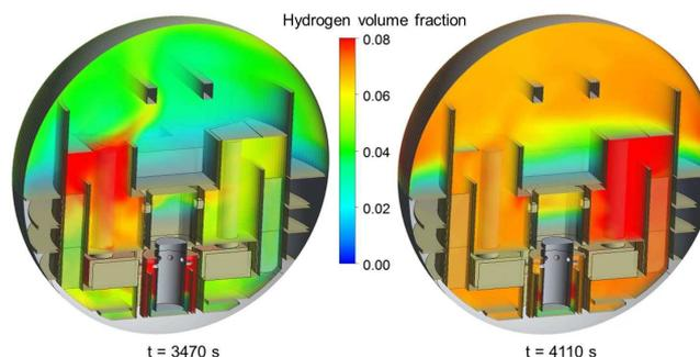
**Figure 4.** Hydrogen distribution in containment at 3470 s (left) and 4110 s (right)
