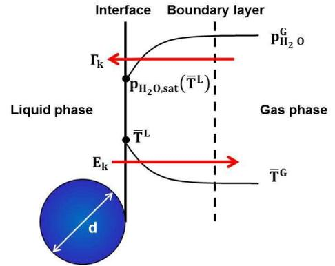
**Figure 2.** Pressure and temperature profiles for a condensing droplet
