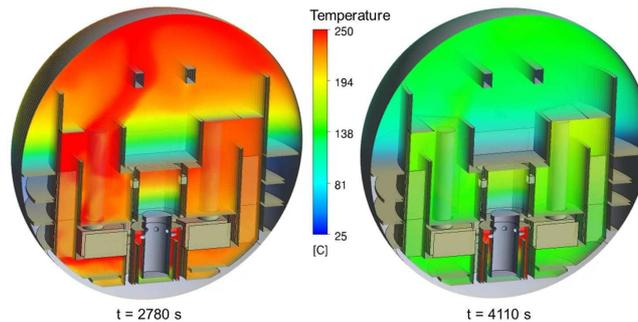
**Figure 5.** Temperature distribution in containment at 2780 s (left) and 4110 s (right)
