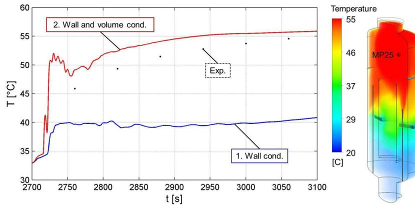
**Figure 3.** Left: comparison of calculated temperature with validation experiment at monitor point MP25; right: temperature distribution of simulation with wall and volume condensation at 3100 s
