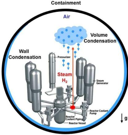
**Figure 1.** Condensation inside containment
