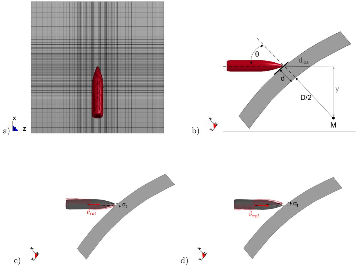
**Figure 1.** Mesh a) and projectile position b) for oblique impact on rounded surface; yaw case A with upper most position c) and case C with lower most position d) shown for  $\theta = 50^\circ$ .
