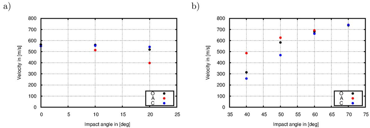
**Figure 2.** Yaw angle influence on projectile after penetration a) and ricochet b) from a rounded surface
