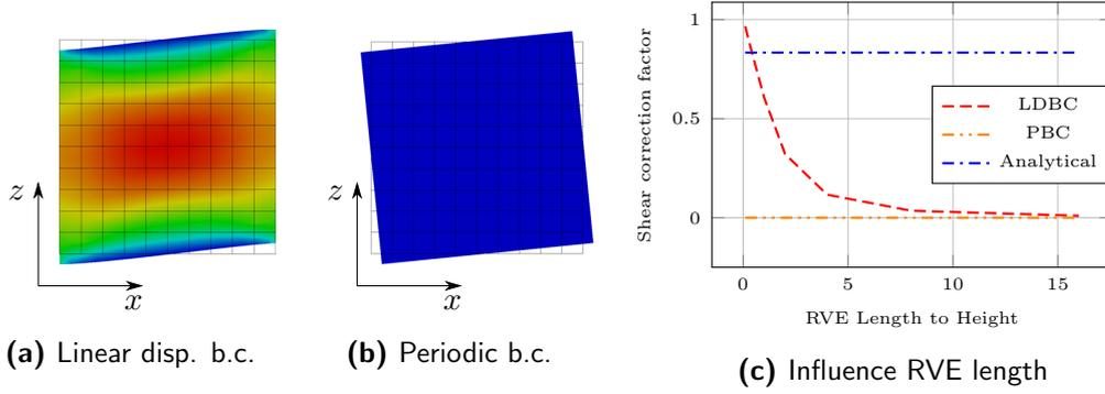
**Figure 1.** Shear deformation of the RVE and length dependency
