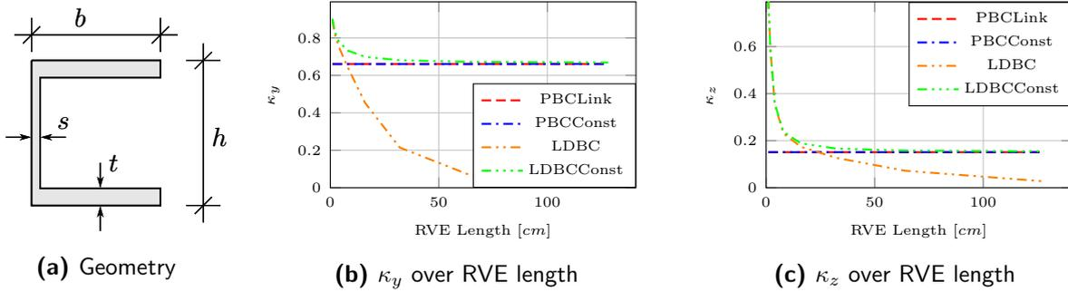
Figure 4. Shear correction factor – U-shaped profile
