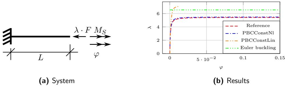
Figure 5. Example – Torsional buckling
