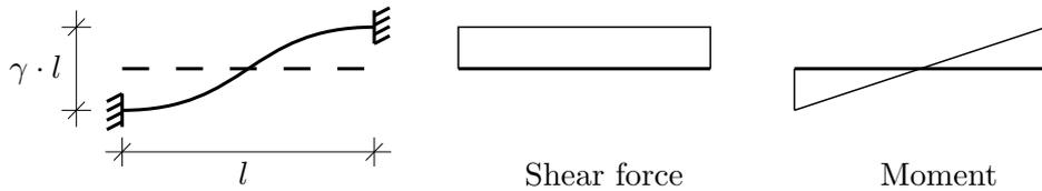
**Figure 2.** Beam shear deformation and stress resultant
