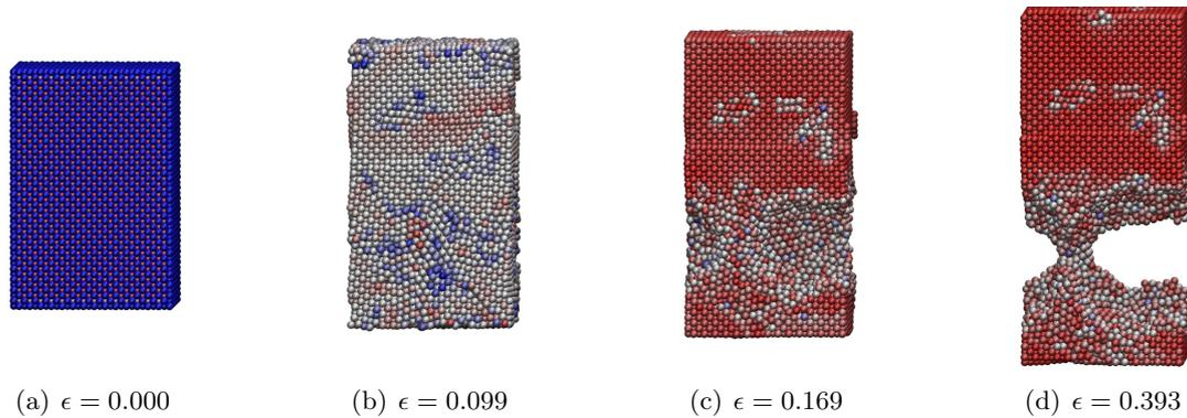
**Figure 2.** Snapshots of several simulation states of a nano-single crystal Al.
