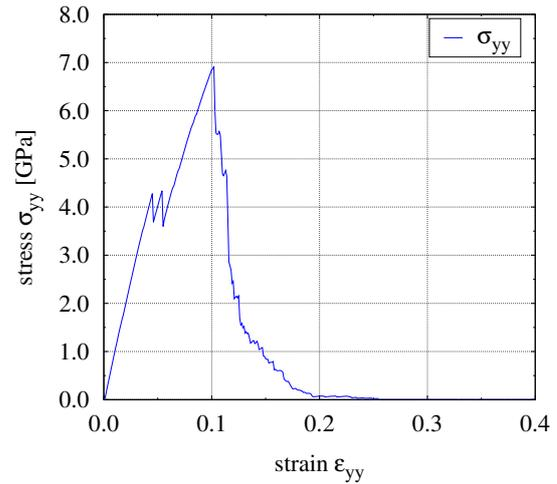
(b) Stress-strain curve polycrystal
