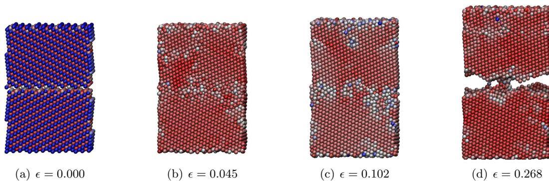
**Figure 3.** Snapshots of several simulation states of a nano-polycrystal Al.
