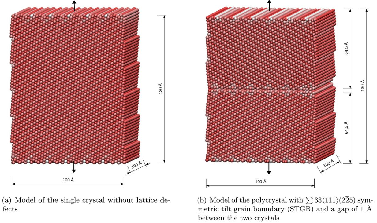
**Figure 1.** Dimensions of the investigated single crystal and polycrystal model
