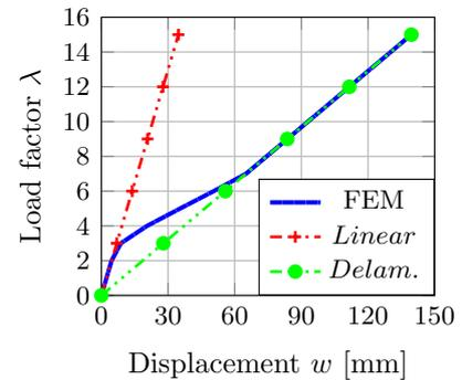
**Figure 10.** Load factor vs. displacement at  $x = L/2$
