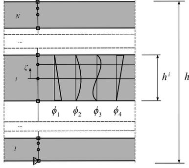
**Figure 1.** Interpolation functions for laminate with N layers
