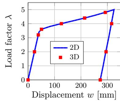
**Figure 7.** Load factor vs. displacement at  $x = 0$
