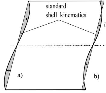
**Figure 2.** a) wrong and b) correct shape of warping displacements
