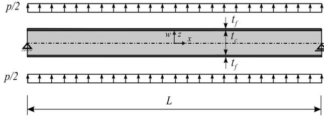
**Figure 3.** Sandwich beam with constant loading
