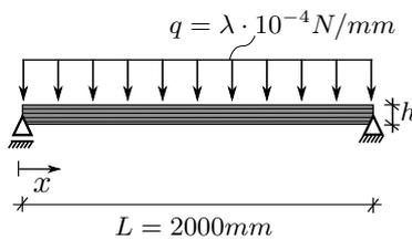
**Figure 8.** Beam with constant loading and  $h = b = 10$  mm
