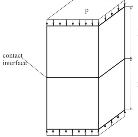
**Figure 3.** Two cubes subjected to uniformly distributed pressure  $p$ , interacting over their common contact interface. Geometry: length  $l = 1$  [m]. Material properties: Young modulus  $E = 2.1 \times 10^5$  [MPa], Poisson's ratio  $\nu = 0.3$ . Loading:  $p = 10$  [MPa].
