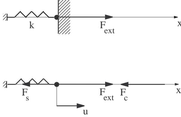
**Figure 1.** Simple one dimensional spring system subject to a single constraint.
