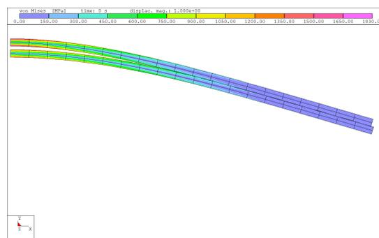
**Figure 6.** The deformed configuration of the beams—contact solution including large displacement.
