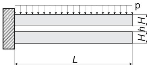
**Figure 4.** Contact of two cantilever beams. Geometry: length  $L = 1000$  [mm], height  $H = 20$  [mm], initial gap  $h = 10$  [mm], thickness  $t = 20$  [mm]. Material properties: Young modulus  $E = 2.1 \times 10^5$  [MPa] and Poisson's ratio  $\nu = 0.3$ . Loading:  $p = 0.5$  [MPa]
