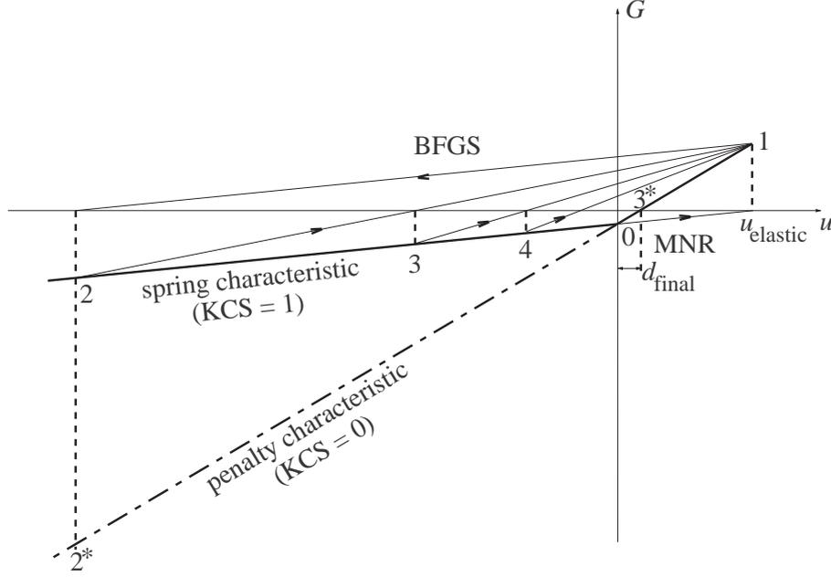
**Figure 2.** The BFGS and MNR iterations for a single degree of freedom system with penalty constraint.
