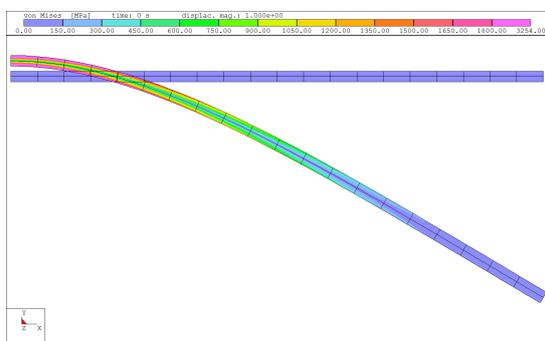
**Figure 5.** The deformed configuration of the beams—initial linear solution.
