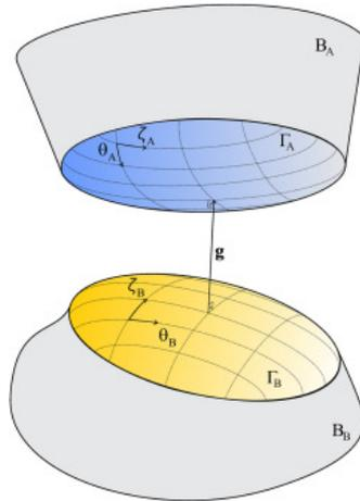
**Figure 1.** Bodies  $B_A$  and  $B_B$  candidate to contact interaction. For each body a subset of the boundary is parameterized: the surfaces  $\Gamma_A$  and  $\Gamma_B$ . (Source: Neto et. al. [8])
