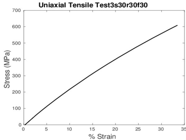
**Figure 3.** Homogenized stress-strain behavior of woven composite subjected to uniaxial tensile loading.
