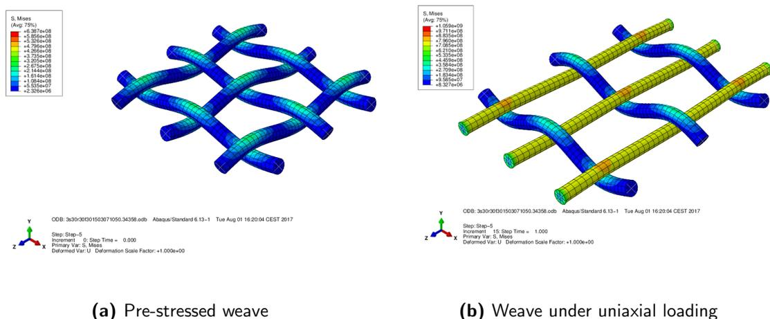
**Figure 2.** Configuration of weaves: Prestressed structure before the uniaxial test (left); Weave subjected to 100% loading
