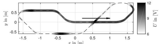
Figure 4. Driving voltage versus track position
