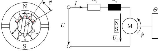
**Figure 1.** Idealized model of a DC motor
