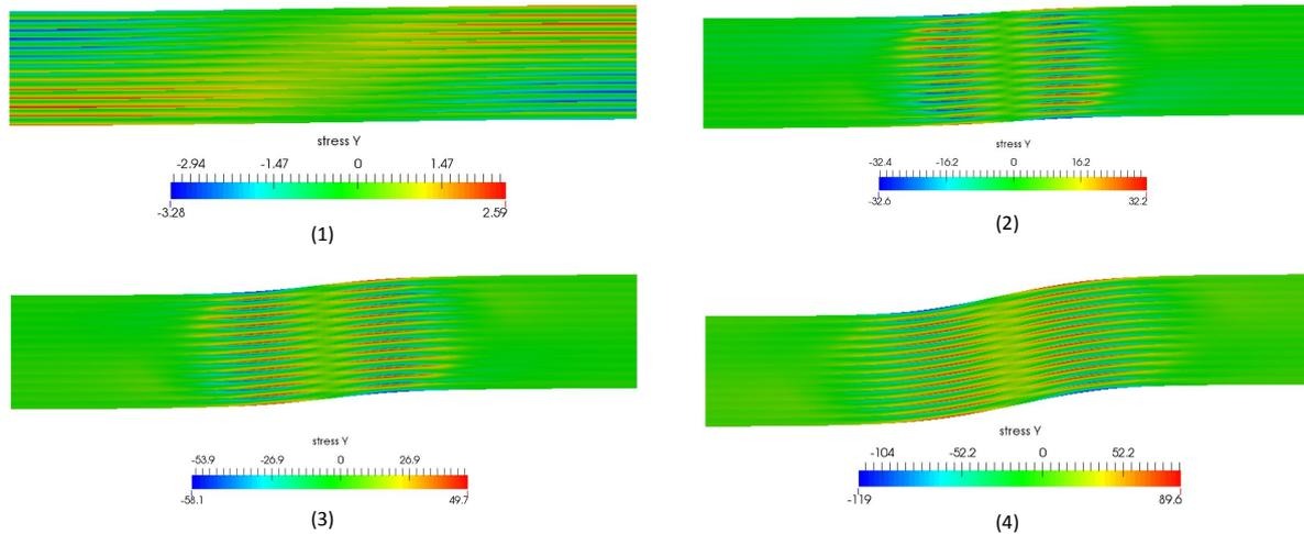
**Figure 4.** Stress distribution in fibers during kink band formation ( $G_{IIc} = 5 \frac{J}{m^2}$ )
