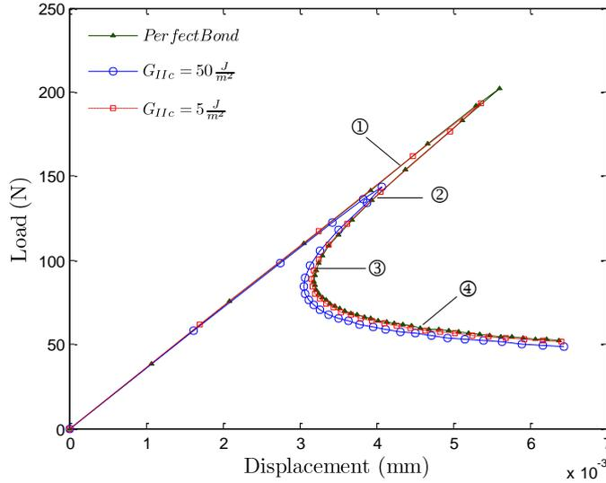
**Figure 3.** Axial load vs. displacement under compressive load
