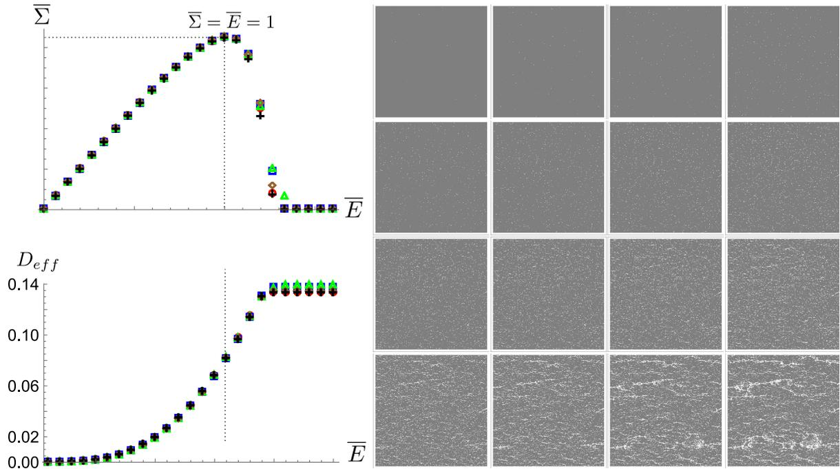
**Figure 3.** Pixel-Erosion simulation of material degradation and diffusion. Left-top: Macroscopic strength normalized stress vs macroscopic strength normalized strain for a specimen under uniaxial tension. Left - bottom: Evolution of the effective diffusivity of the material during material degradation (the colored symbols correspond to the 5 random realizations). Right: Evolution of microcracking in the specimen subject to tension up to localization.
