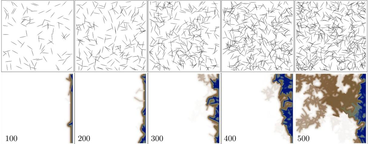
**Figure 1.** Pixel-FE simulation of diffusion in a porous specimens of size  $1\text{cm} \times 1\text{cm}$  with 100, 200, 300, 400 and 500 microcracks of length  $1000\mu\text{m}$  and width  $25\mu\text{m}$ . Upper row: morphology of the microcracked material. Lower row: depth of ingress of a diffusing species in all the specimens after a certain period of time
