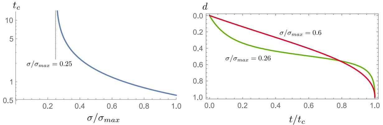
**Figure 2.** Left: Critical time to failure  $t_c$  vs the applied stress level  $\frac{\sigma}{\sigma_{max}}$ . Right: Evolution of damage  $d$  as a function of the normalized time to failure
